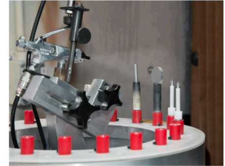
Spraying \text{MoS}_2 mixed with polymer binder
