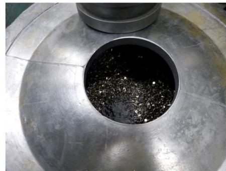
Parts tumbled in drum with \text{MoS}_2
