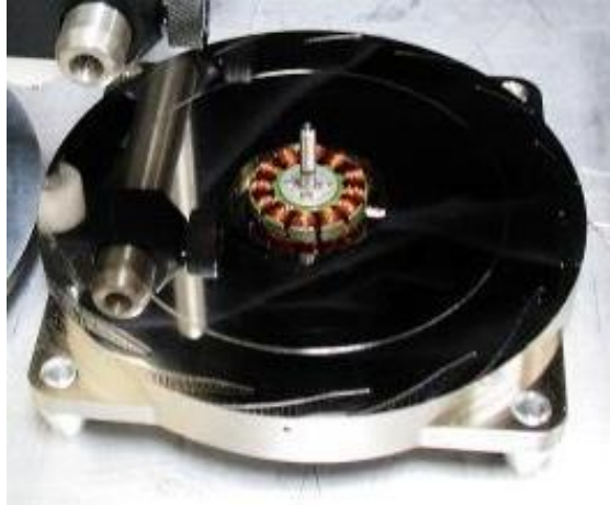
Figure 123. V5 baseplate with new spiral groove pattern.
