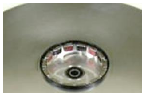
Figure 14. Motor rotor magnet array, flux ring and bearing integrated into impeller platen.
