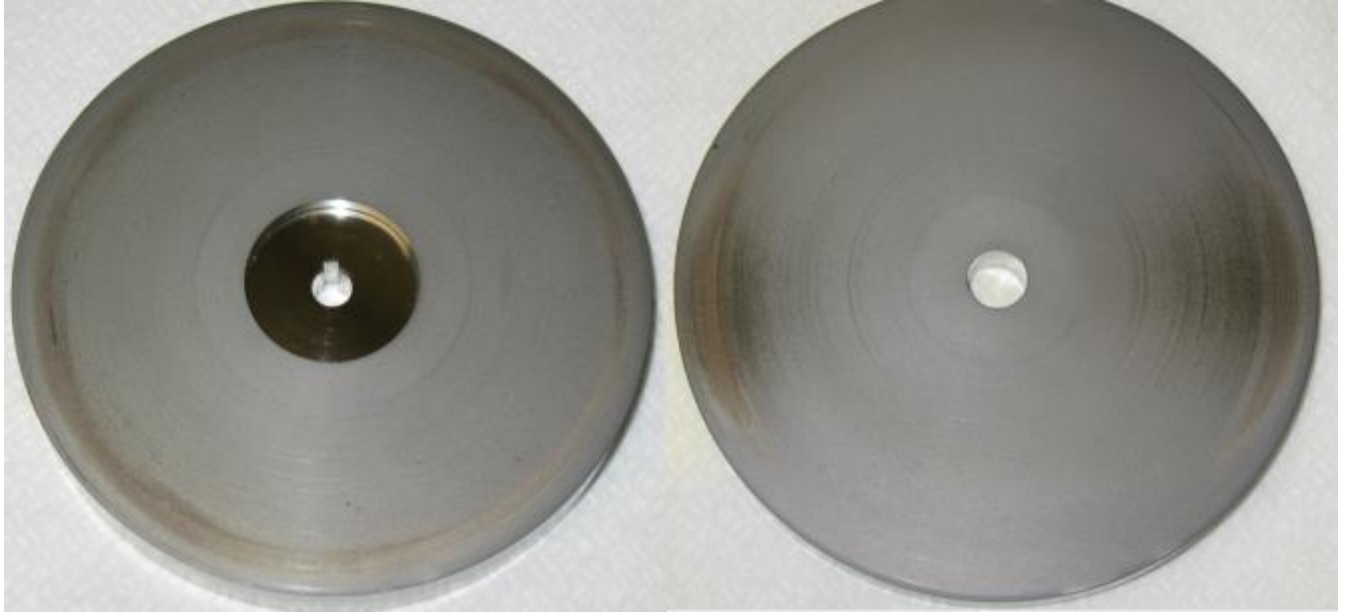
Figure 143: Wear patterns of substitute impeller (left) and baseplate (right).
