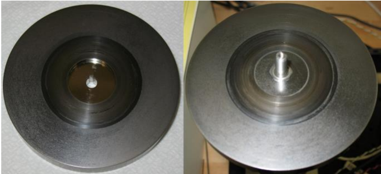
Figure 145: Parts coated using standard deposition, after 16 hours at 1000rpm.
