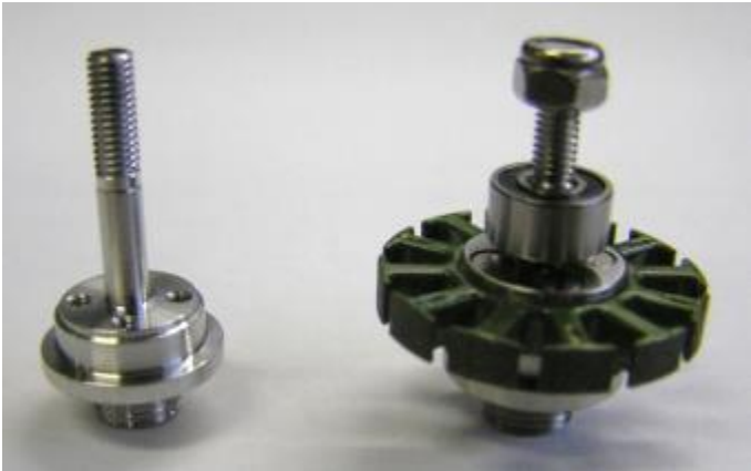
Figure 116. New motor stator mount and shaft.
